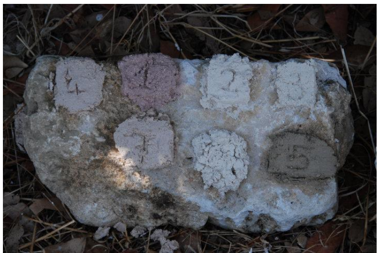
Figure 17. Lime mortar colour tests.
